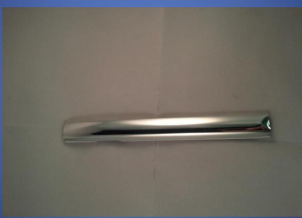
Result of the test of alkaline resistance FIAT 9.57448. Piece sealed with Superseal process (no visible attack)
