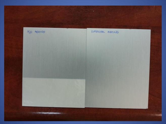
Result of the test of alkaline resistance GMW14665 at pH 13,5. Comparison between a piece sealed with conventional sealing (left) and one sealed with Superseal (right)
