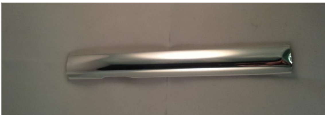
Figure 1: Result of the test of alkaline resistance FIAT 9.57448. Piece sealed with Superseal process (no visible attack).
