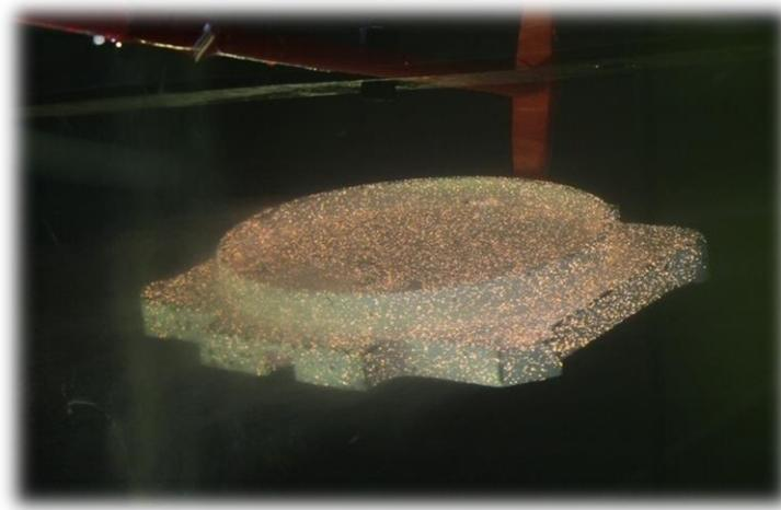
Distinctive feature of the process is participation the micro arc discharges in the coating formation process. As result composition and structure of the MAO-coatings differ from anodic coatings essentially.
